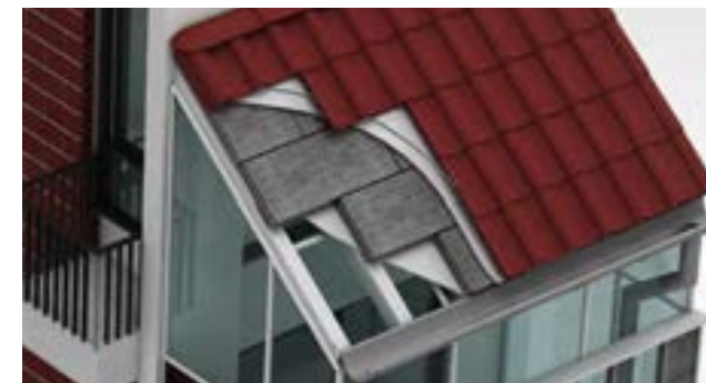
Pitched Roof Insulation Suggested Product: STYRO Graypor 380
