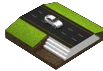
Road Construction Over Poor Soils
