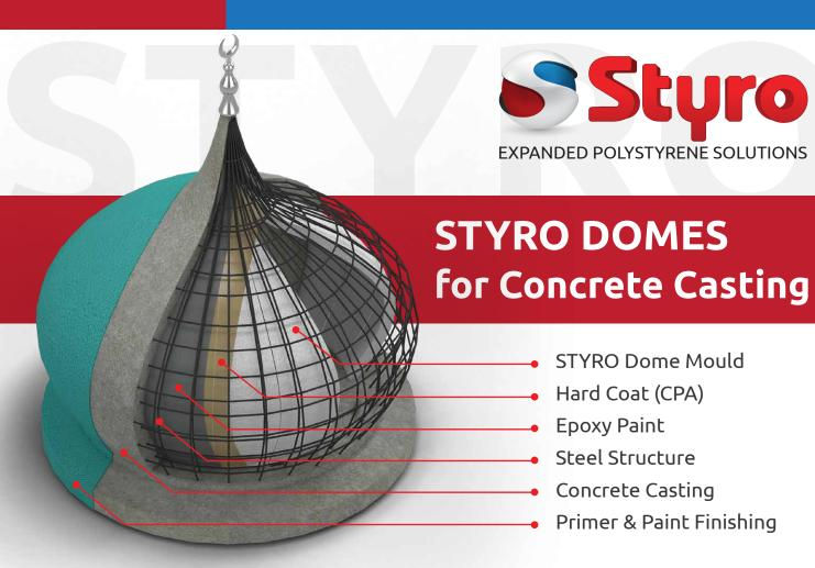
STYRO Dome is used as a mould for concrete casting which became popular in all construction applications across the globe. STYRO Domes can be easily molded into any shape and size, this flexability makes STYRO Products the ideal solution for wide range of construction and art projects.
