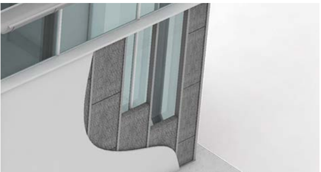
Insulation Behind Curtain Walls Suggested Product: STYRO Graypor 220
