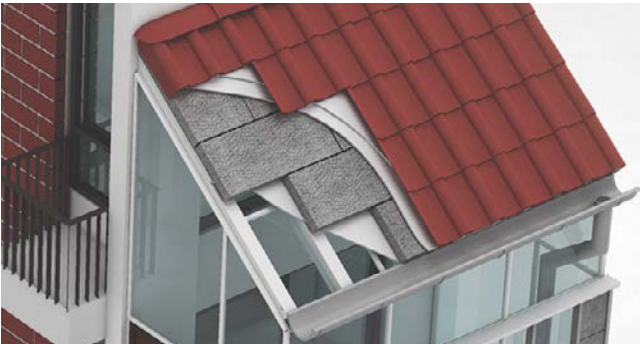
Pitched Roof Insulation Suggested Product: STYRO Graypor 380
